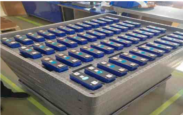
Battery cell’s collar containers + EPP foam solution
